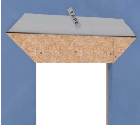
STEP 5 Temporarily secure WRB above the header exposing the substrate.
